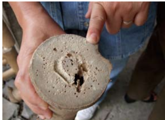
Section of an untreated bamboo culm with insect damage. La Union Province, May 28, 2007.
